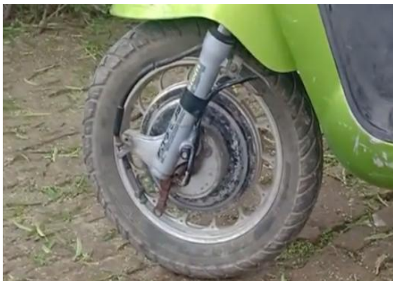
Fig. 4: Real time photo BLDC hub motor on front Wheel of scooty.
